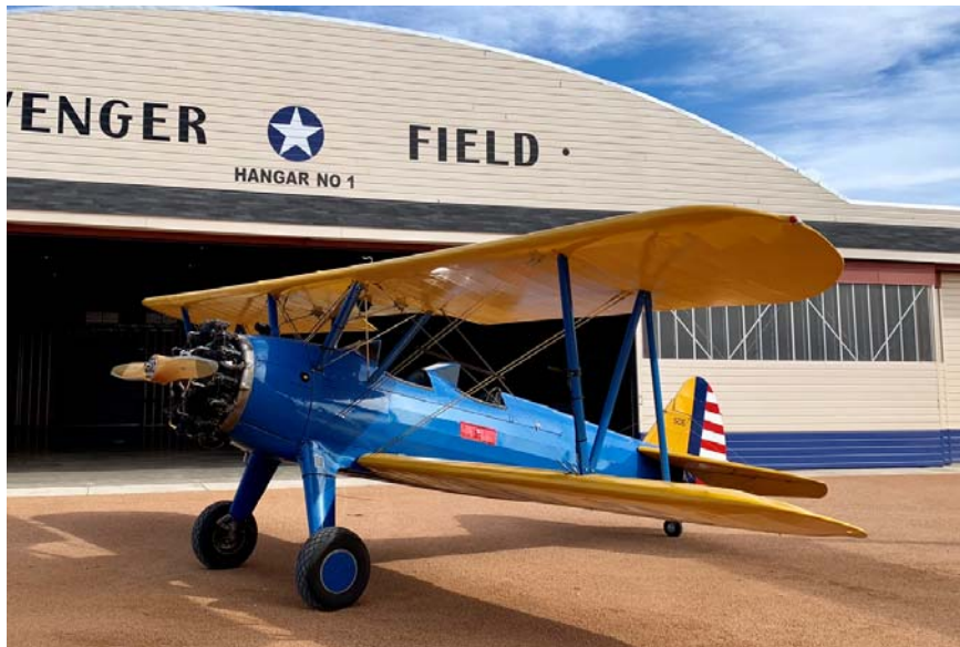
Boeing Stearman Kaydet - Primary Trainer Aircraft Flown by WASP Pilots - Cont. Pg. 23
