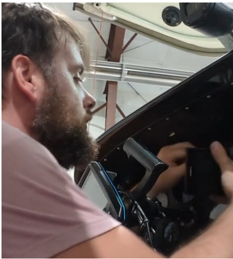
Above: On step and on to great adventures. Left: Hands-on in the cramped cockpit: upgrading Ruth Bader Wingsburg's panel. A full panel modernization—new GPS, G5s, radios, and rewiring—turned the author's Lake 200EP into a capable and practical IFR platform.
