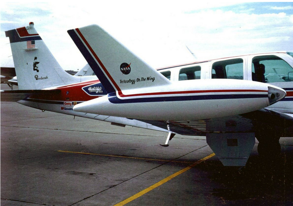
Close-up view of the winglet (1980-81) before winglets had been adopted by general aviation, and the first flown around the world. "Worth their weight in fuel," says Cal.
