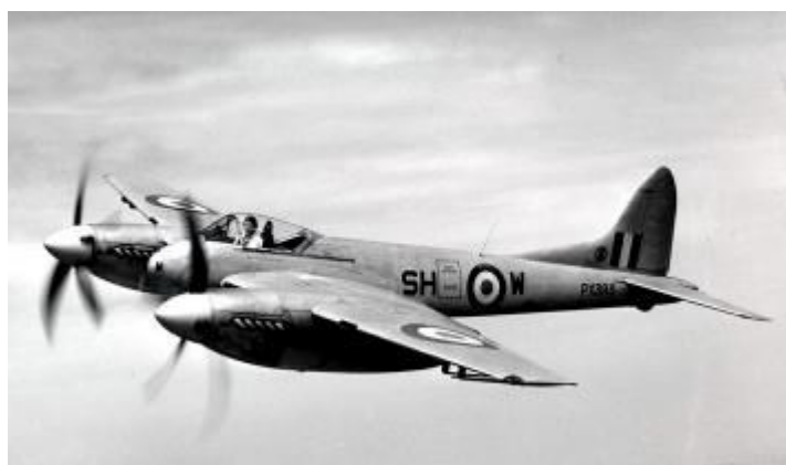
Top: The only flight of the Hughes H-4 Hercules “Flying Boat,” 400,000 pounds of airplane, made of Wisconsin birch trees. The de Havilland Hornet was made of Marshfield plywood and remained in service with the RAF until 1956.
