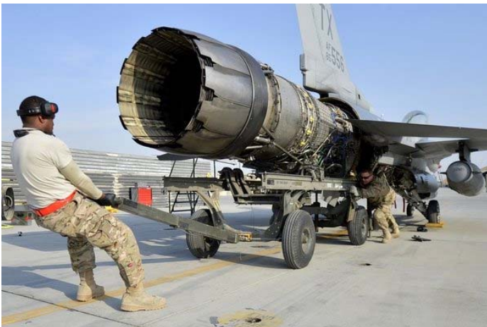
F-16 Falcon Engine Removal "Pulling the Pusher"
