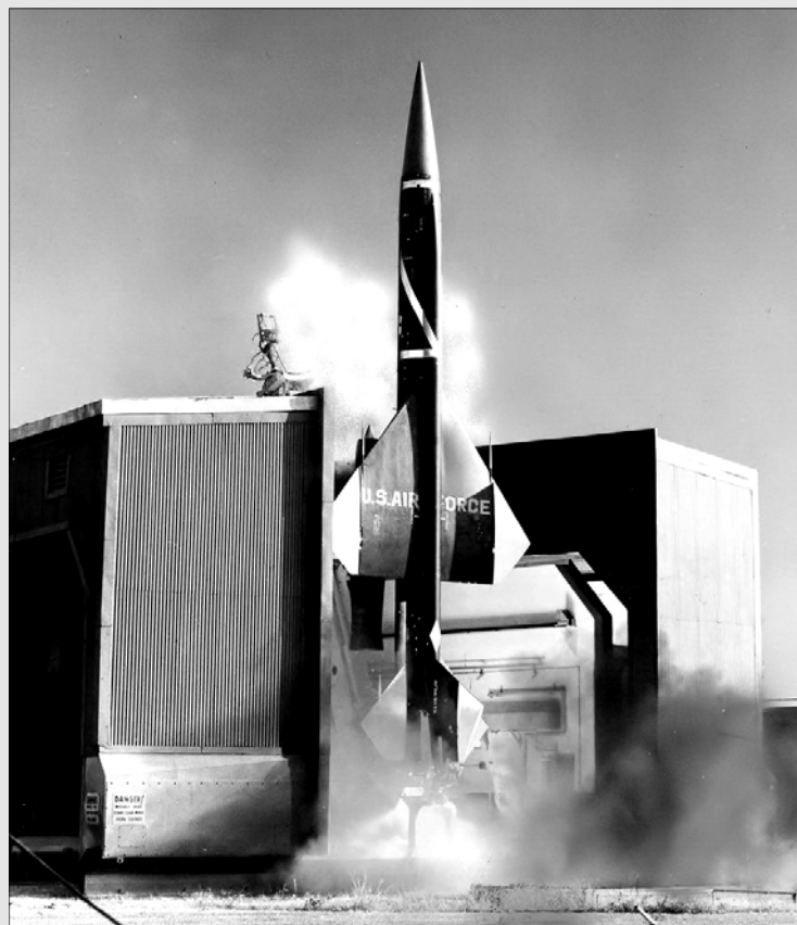
A BOMARC test launch. Just prior to launch, the two hangar halves slid apart and a launch rail raised the missile to the vertical. U.S. Air Force photo.
