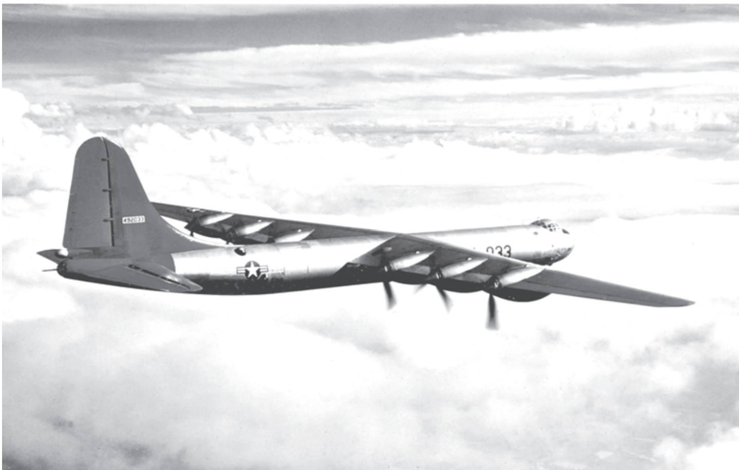
The Convair B-36B, the largest operational bomber ever built. The B-36 had an un-refueled range of more than 10,000 miles, and on the Schreier mission carried a crew of 17.
